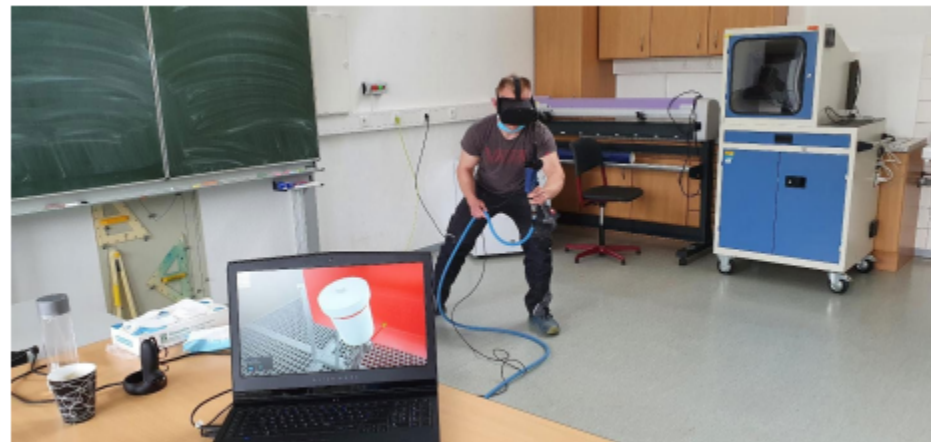
Fig. 1 Apprentice learning with the VR-based painting simulator
